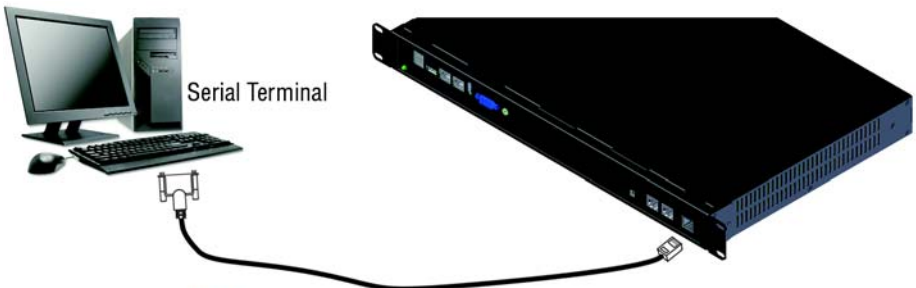
Figure 8. Connecting a serial terminal with RJ45 to DB-9 adapter
